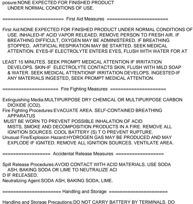
Handling and Storage Precautions:DO NOT CARRY BATTERY BY TERMINALS. DO NOT DROP BATTERY, PUNCTURE OR ATTEMPT TO OPEN BATTERY CASE. KEEP AWAY FROM FLAMES DURING AND IMMEDIATELY AFTER CHARGE. AVOID PROLONGED OVERCHARGES IN CONFINED ARE AS. STORE AT AMBIENT ROOM TEMPERATURE. DO NOT SUBJECT PRODUCT TO OPEN FLAME OR FIRE. Other Precautions:AVOID CONDITIO
